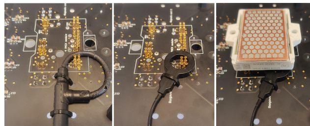
Figure 11. Mounting Detail Rogowski Coil to PCB
