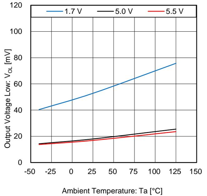
Figure 6. Output Voltage Low vs Ambient Temperature ( $I_{OUT} = 1\text{ mA}$ )
