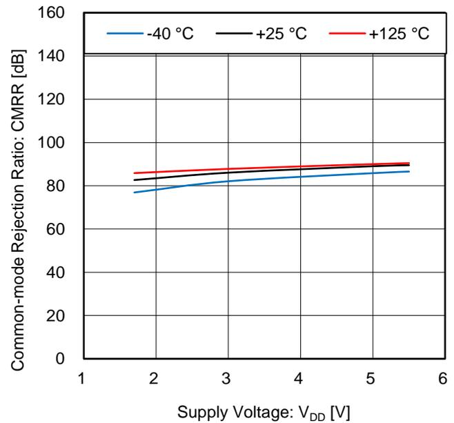
Figure 16. Common-mode Rejection Ratio vs Supply Voltage
