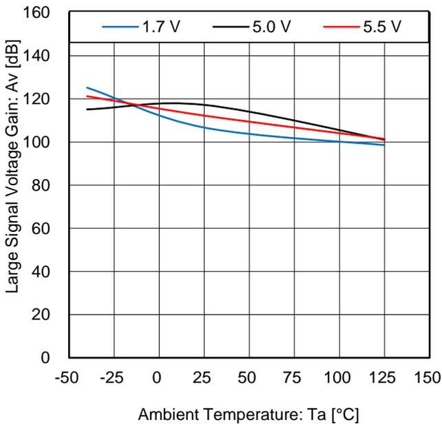
Figure 15. Large Signal Voltage Gain vs Ambient Temperature
