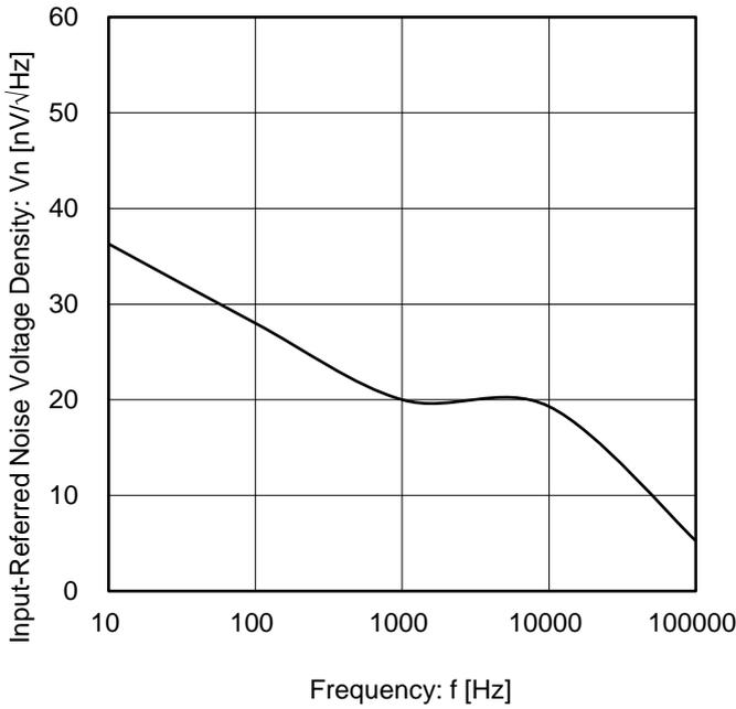
Figure 21. Input-Referred Noise Voltage Density vs Frequency ( $V_{DD} = 5\text{ V}$ )
