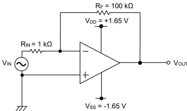
$$V_{OUT} = -\frac{R_F}{R_{IN}} V_{IN}$$
