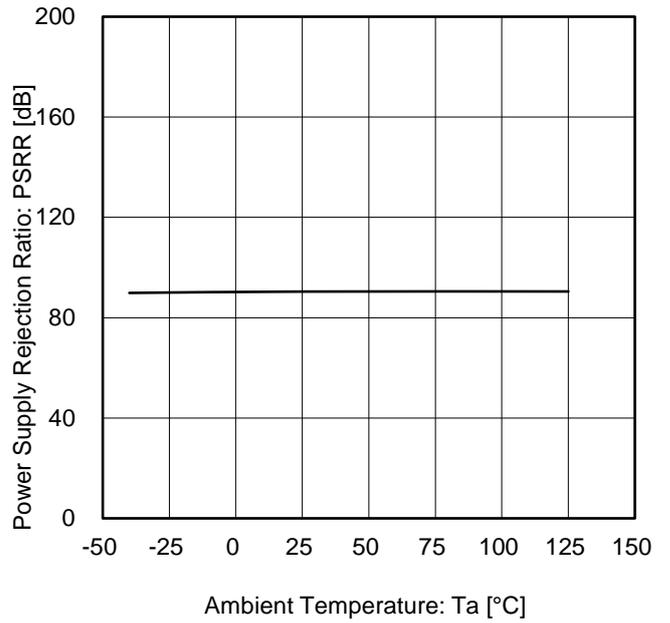
Figure 18. Power Supply Rejection Ratio vs Ambient Temperature
