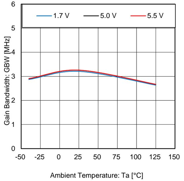
Figure 22. Gain Bandwidth vs Ambient Temperature
