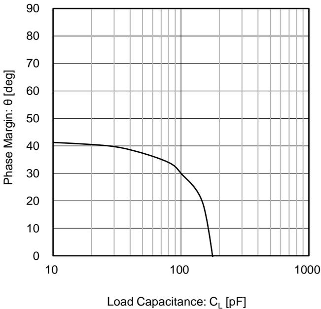
Figure 23. Phase Margin vs Load Capacitance ( $V_{DD} = 5\text{ V}$ ,  $G = 40\text{ dB}$ )
