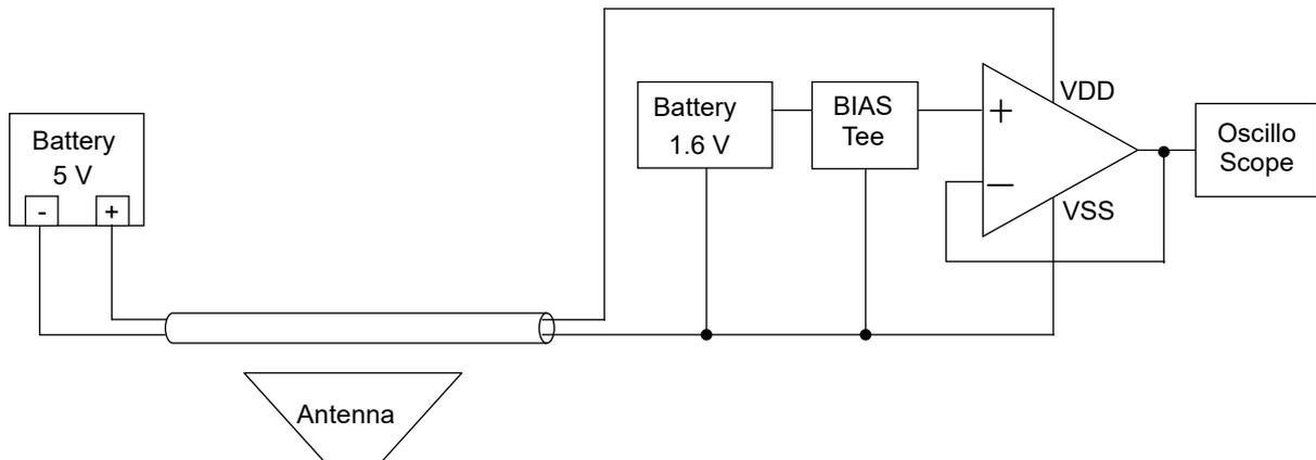
Figure 26. Measurement Circuit of EMI Evaluation
