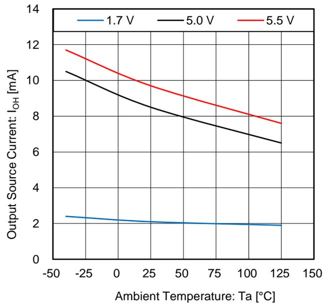
Figure 8. Output Source Current vs Ambient Temperature ( $V_{OUT} = V_{DD} - 0.4\text{ V}$ )
