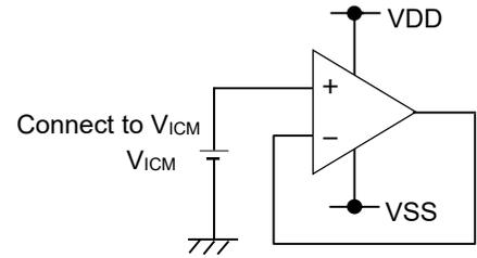
Figure 27. Example of application unused circuit processing
