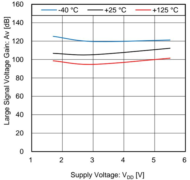
Figure 14. Large Signal Voltage Gain vs Supply Voltage
