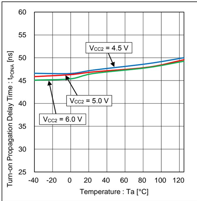
Figure 17. Turn-on Propagation Delay Time vs Temperature (INA = PWM, INB = L)
