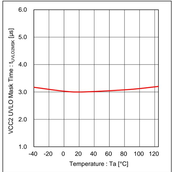
Figure 24. VCC2 UVLO Mask Time vs Temperature
