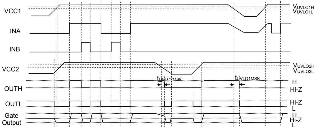
Figure 27. Input-Output Timing Chart
