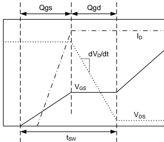
Figure 30. Gate Charging Characteristics of Power Devices
