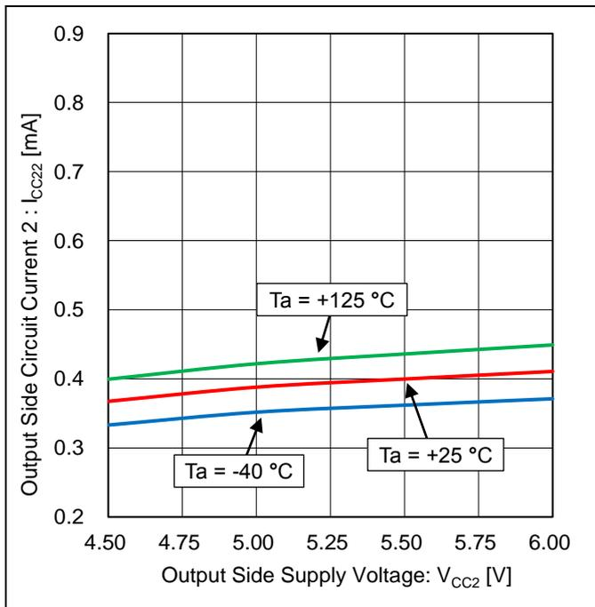
Figure 9. Output Side Circuit Current 2 vs Output Side Supply Voltage (OUT = H)
