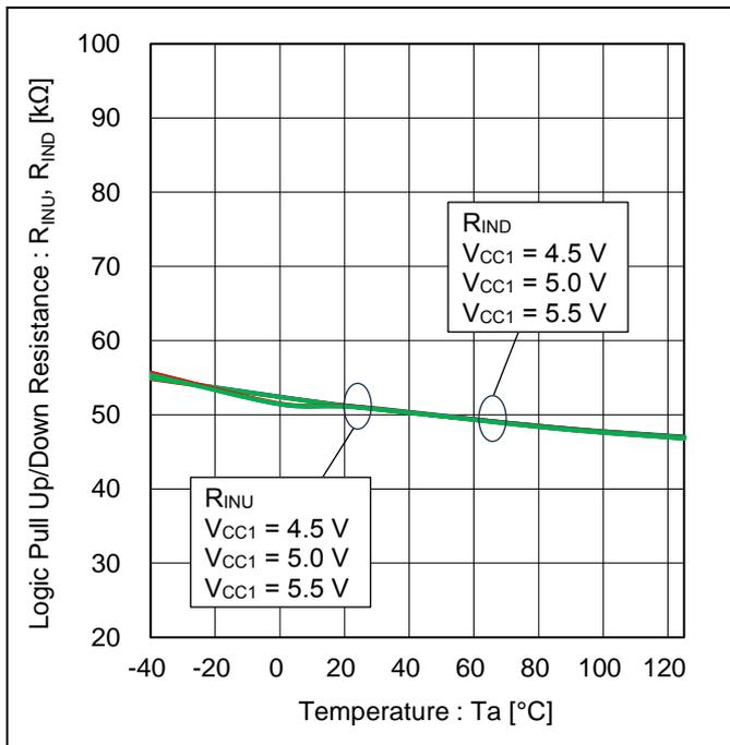
Figure 13. Logic Pull Up/Pull Down Resistance vs Temperature
