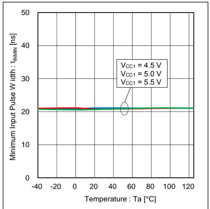
Figure 14. Minimum Input Pulse Width vs Temperature
