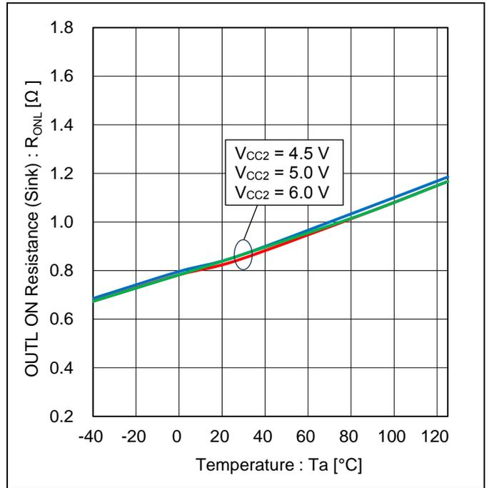
Figure 16. OUTL ON Resistance (Sink) vs Temperature
