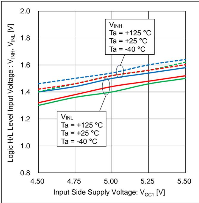
Figure 11. Logic (INA/INB) H/L Level Input Voltage vs Input Side Supply Voltage
