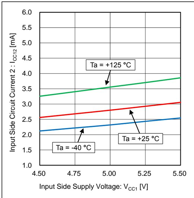
Figure 5. Input Side Circuit Current 2 vs Input Side Supply Voltage
