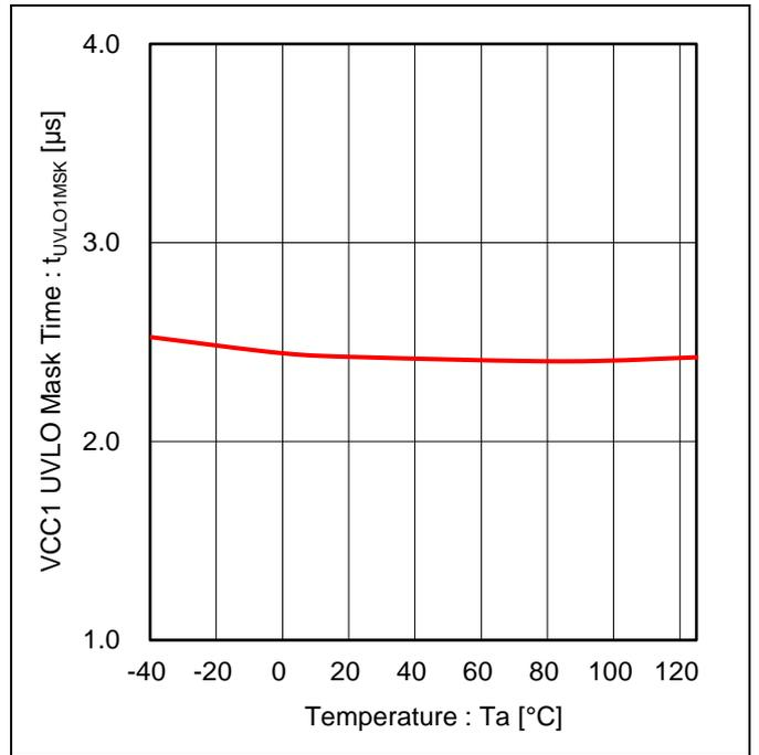
Figure 22. VCC1 UVLO Mask Time vs Temperature
