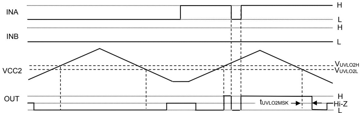
Figure 26. Output Side UVLO Function Operation Timing Chart
