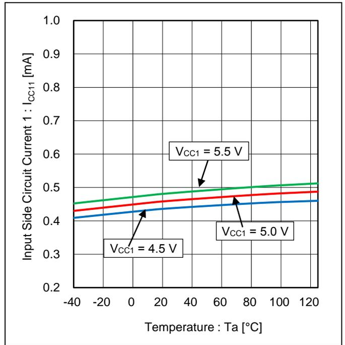
Figure 4. Input Side Circuit Current 1 vs Temperature
