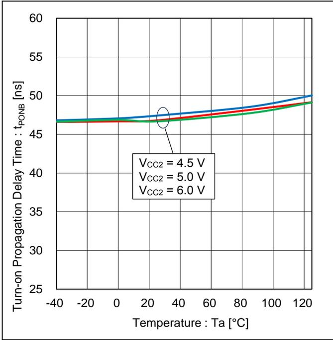
Figure 19. Turn-on Propagation Delay Time vs Temperature (INA = H, INB = PWM)
