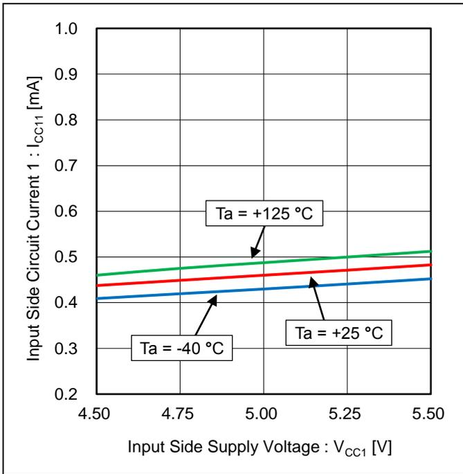
Figure 3. Input Side Circuit Current 1 vs Input Side Supply Voltage
