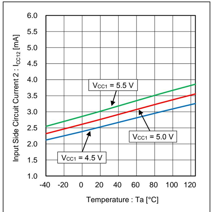
Figure 6. Input Side Circuit Current 2 vs Temperature
