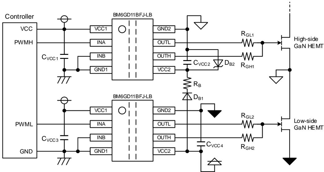
Figure 28. GaN HEMT Drive Application Circuit (Half-bridge configuration)
