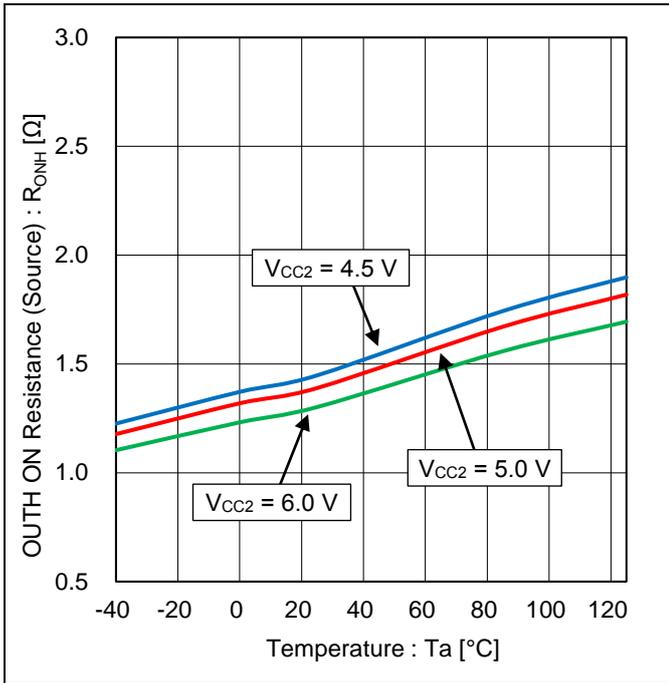
Figure 15. OUTH ON Resistance (Source) vs Temperature
