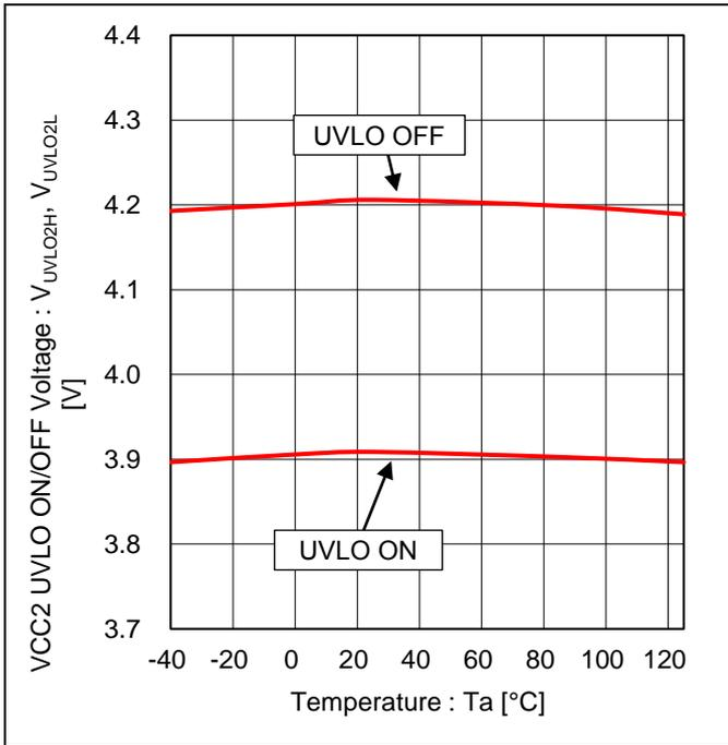
Figure 23. VCC2 UVLO ON/OFF Voltage vs Temperature
