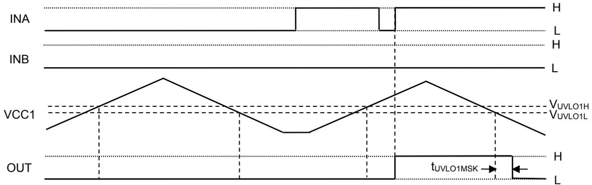
Figure 25. Input Side UVLO Function Operation Timing Chart
