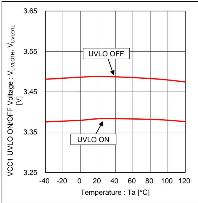
Figure 21. VCC1 UVLO ON/OFF Voltage vs Temperature
