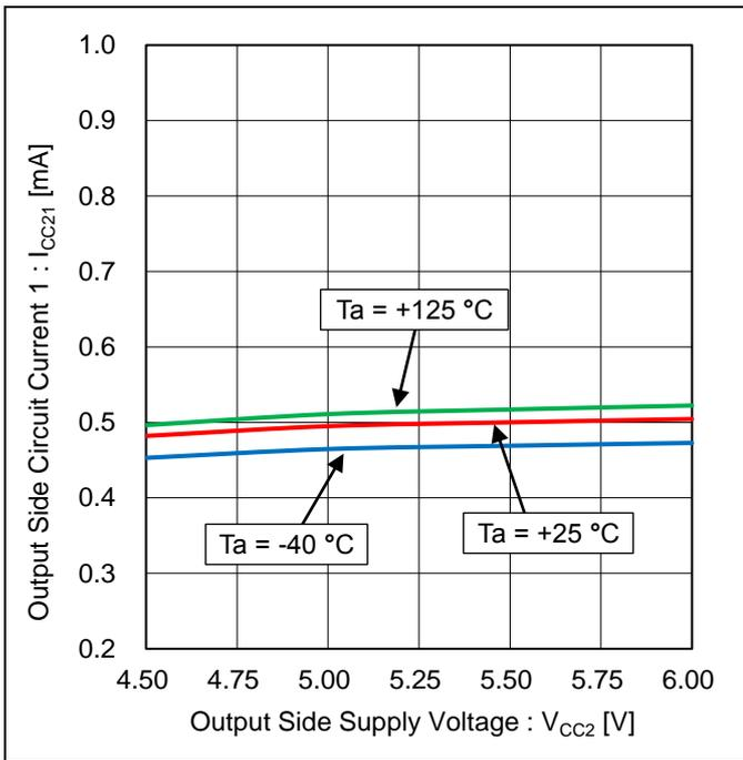
Figure 7. Output Side Circuit Current 1 vs Output Side Supply Voltage (OUT = L)
