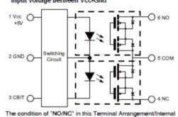
Connections (Top View) Input 5V DC between Vcc-Gnd.
