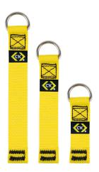
Features & Benefits Terminated steel D-ring with reinforced stitching for secure tool attachment  $\sim$  Dynamic load tested (1:1 safety factor)  $\sim$  Sizes: 100, 150, and 200mm  $\sim$  Conforms to ANSI/ISEA 121-2018  $\sim$  Max load: 4kg
