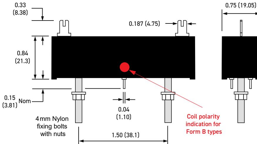
**Important:** For all Form B types, the correct coil polarity must be observed. The positive connection is shown by the red spot on the package.
