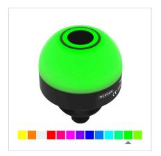
K50 Pro: Pick-IQ Adjustable-Field Sensor 10-30 V dc; Polycarbonate; IP66, IP67, IP69K Input: Modbus; Colors: Multicolor 4-pin M12 Integral QD
