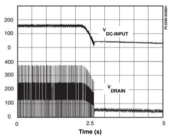
Figure 13. Slow Power-down Timing With Optional External (4 M $\Omega$ ) UV Resistor Connected to EN/UV Pin.
