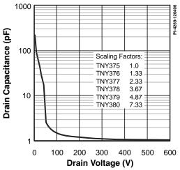
Figure 26.  $C_{\rm oss}$  vs. Drain Voltage.
