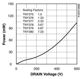
Figure 27. Drain Capacitance Power.
