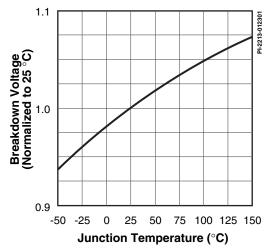
Figure 21. Breakdown vs. Temperature.
