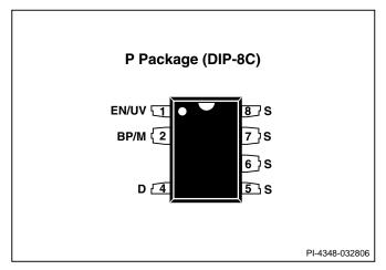
Figure 3. Pin Configuration.
