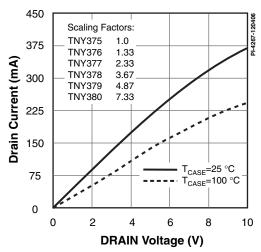
Figure 25. Output Characteristics.
