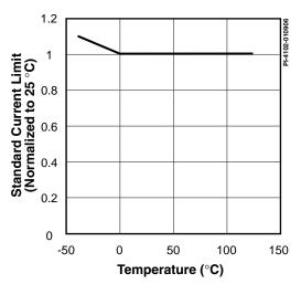
Figure 23. Standard Current Limit vs. Temperature.
