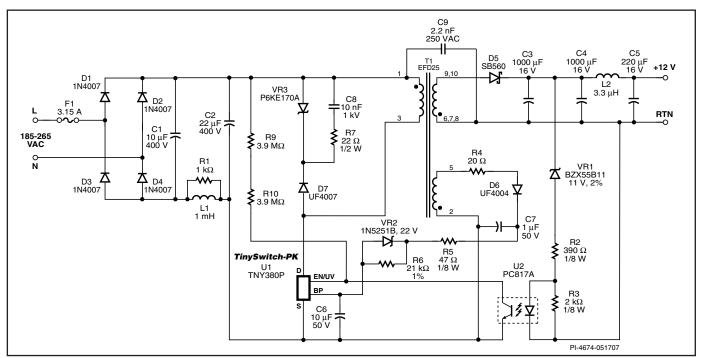
Figure 15. Single 230 VAC Input 20 W Continuous and 45 W Peak Power Supply Using TNY380P.
