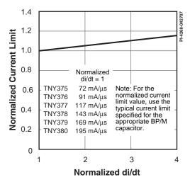
Figure 24. Current Limit vs. di/dt.
