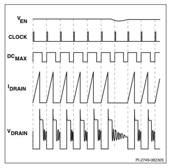
Figure 6. Operation at Near Maximum Loading (f<sub>osc</sub> 264 kHz).
