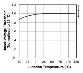
Figure 28. Undervoltage Threshold vs. Temperature.
