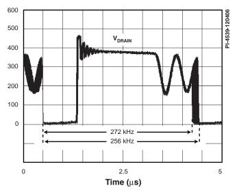
Figure 4. Frequency Jitter.
