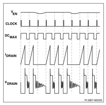
Figure 7. Operation at Moderately Heavy Loading (f<sub>osc</sub> 264 kHz).
