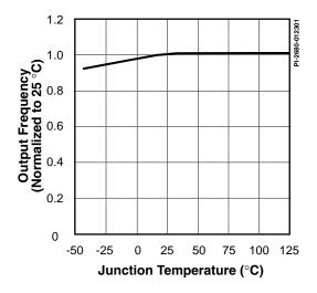
Figure 22. Frequency vs. Temperature.
