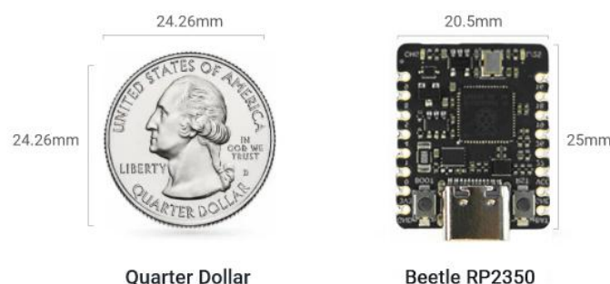
Coin-sized development board - Beetle RP2350
