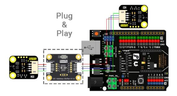
Figure: Wiring Diagram of I2C Address Shifter, sensors and Arduino UNO
