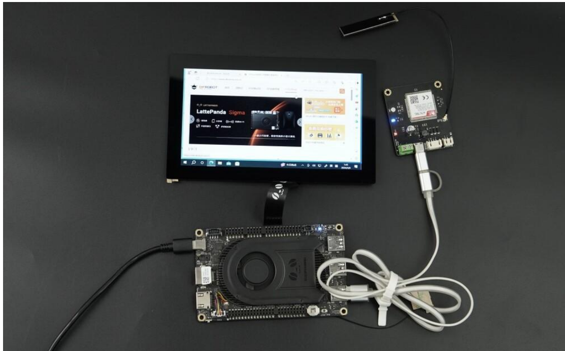
Connection Diagram of CAT1 A7670G 4G Communication Module and LattePanda 3 Delta single board computer
