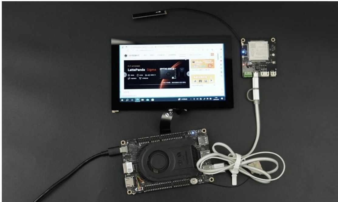
Connection Diagram of 4G CAT1 communication module and LattePanda 3 Delta single board computer
