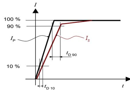
Figure 6:  $t_{D10}$  (delay time @ 10 %) and  $t_{D90}$  (delay time @ 90 %)
