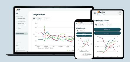
With the online data loggers connected to the testo Saveris Cloud, your indoor climate monitoring takes place effortlessly in the background. You don't have to do anything yourself – the process is fully automated. You can access all measurement data in the cloud via smartphone, tablet or PC. All you need is a valid license and to set up the system once: configure the online data loggers and set limit alarms. The rest takes care of itself.
