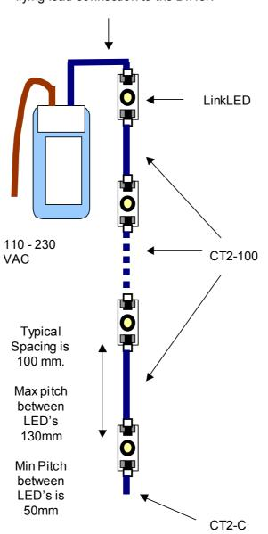
CT2-100 with one connector cut off to make a flying lead connection to the Driver.
