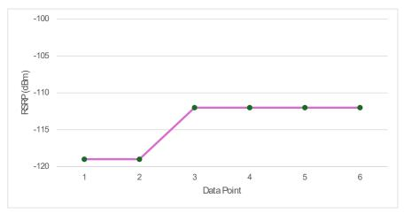
An RSRP value of -120 dBm is generally the recognized minimum requirement suitable for the data rates of SMS, CAT-1, CAT-1 Bis connectivity.
