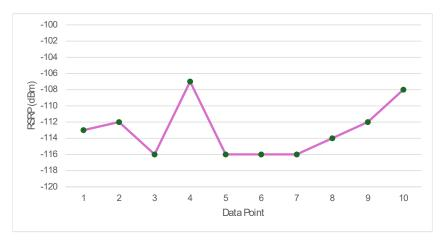
An RSRP value of -120 dBm is generally the recognized minimum requirement suitable for the data rates of SMS, CAT-1, CAT-1 Bis connectivity.
