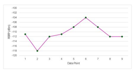
An RSRP value of -120 dBm is generally the recognized minimum requirement suitable for SMS connectivity.
