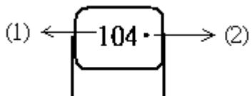
(1) Rated capacitance: Identified by 3-figure code.
