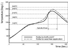
Infrared soldering profile
