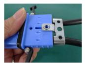
Insert M4 screw through spring washer, fixing sheet and housing, also aim it to the M4 nut on back side and use the screwdriver to fasten it.
