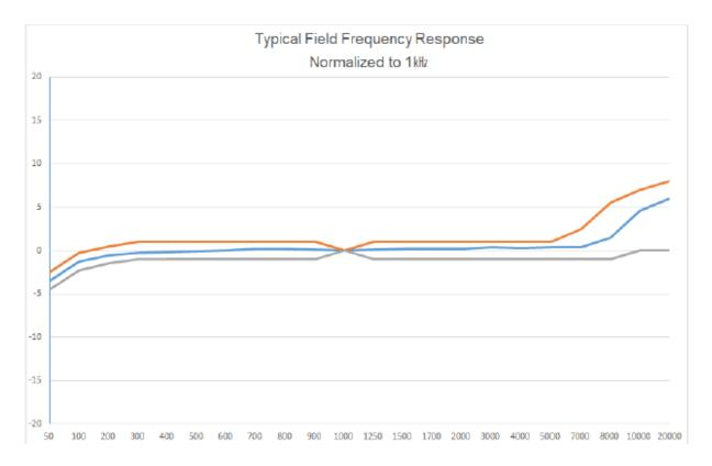
TEST CONDITION: 23±2°C, 65±20% R.H., Typical specifications are measured at VDD = 1.8V Speaker: 1Pa (94dBSPL@1klb) at 50cm distance from a loud-speaker
