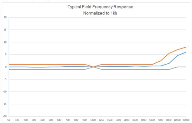
TEST CONDITIONS: 23±2°C, 65±20% R.H., Typical specifications are measured at VDD = 1.8V Speaker: 1Pa (94dBSPL@1kHz) at 50cm distance from a loud-speaker
