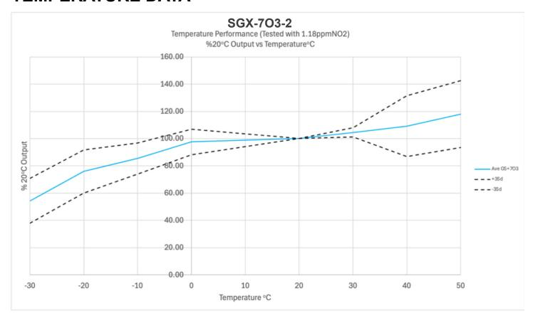
Note: the output of the SGX-7O3-2 sensor is of a negative polarity compared to CO or H2S for example.
