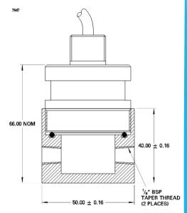
The Flow Cap allows the IR600 to be used in applications where it is to be aspirated permanently with a pumped or pressurised sample. The cap is made of 316 stainless steel and can be used in a variety of applications involving pumped sampling analysis or detection systems.
