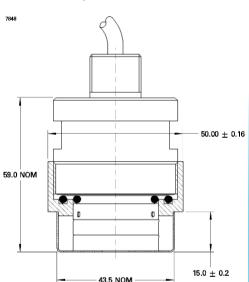
The Weather Cap protects the IR600 from water when used in external locations, where rain or spray could interfere with the safe working of the head, or in internal locations where water jets, sprays or hoses are used routinely for cleaning purposes, etc. The cap is made of 316 stainless steel and has been tested to IP64 for effectiveness, and also to ensure that it does not significantly affect the IR600's performance.
