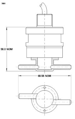
The Quick Calibration Hood is constructed from polypropylene, and provides a convenient means of supplying test gases to the IR600 in the field, for calibration and checking purposes. The assembly push-fits into the central gas access recess of the head, and is designed to accommodate 6 mm ID or ¼" flexible tubing.
