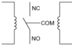
3. Current Flows In the Other Coil (NC Position)
