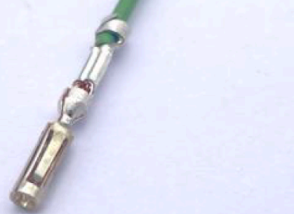
Terminal Sample from new capacity tooling. Localized gold plating is present on terminal beams as defined in product drawing 770520.
