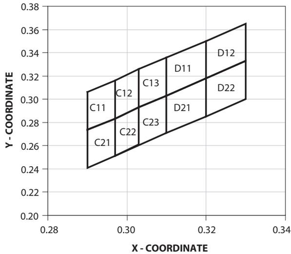
Figure 1. White binning in CIE 1931 Chromaticity Diagram.
