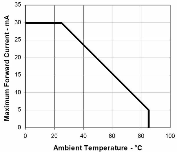
Figure 4. Maximum forward current vs. ambient temperature
