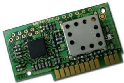
This module enables a **two-ways digital link** up to a range of **6000m**.
