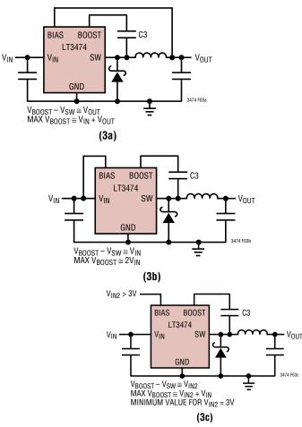
Figure 3. Generating the Boost Voltage
