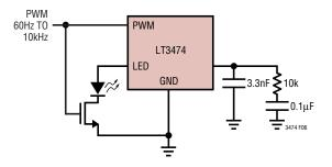
Figure 6. Dimming Using PWM Signal
