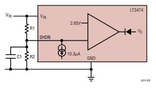
Figure 2. Undervoltage Lockout
