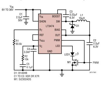
Step-Down 1A LED Driver with PWM Dimming
