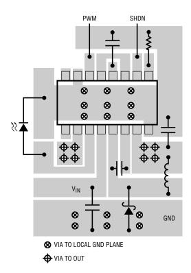
Figure 7. Recommended Component Placement
