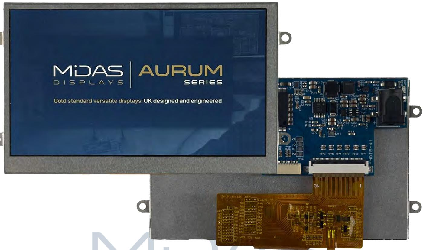
The module integrates a high-brightness TFT panel with a dedicated HDMI interface board, providing a ready-to-use display solution for embedded, industrial, and commercial applications. Designed for ease of integration, the module accepts a single 5–12 V supply and directly converts HDMI input signals to the required RGB interface for the display.
