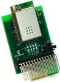
The ZeroG 802.11 PICtail Plus Daughter Board is a demonstration board for evaluating Wi-Fi connectivity using PIC microcontrollers and the ZeroG ZG2100M module.
