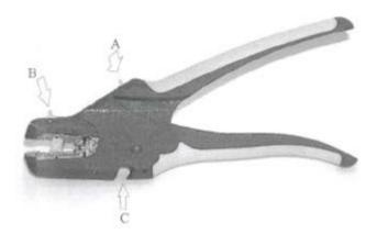
The D01627 has been designed to remove insulation from wire and cables, ideal for installation electricians. The design of the tool enables the user to strip cable of 6mm<sup>2</sup> (10AWG) down to 0.08<sup>2</sup> (27AWG) with an easy action gripping pad adjuster (A) and blade depth adjuster (B); providing in the one tool what was previously only available by having several. The tool also has a cut off blade (C) handling cable up to 6mm<sup>2</sup> (10AWG) stranded copper conductor.
