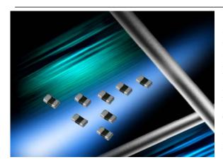
AVX 0201 Multi-Layer Varistors are designed for circuits where board space is a premium. 0201 MLV offer bi-directional ESD protection in the smallest package available. The added advantage is EMI/RFI attenuation. 0201 MLV can replace 2 diodes and the EMC capacitor for a one chip solution.
