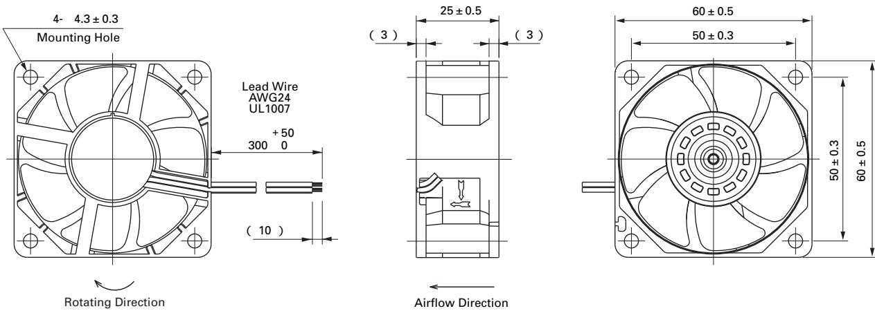
**Reference dimension of mounting holes and vent opening** (unit : mm)
