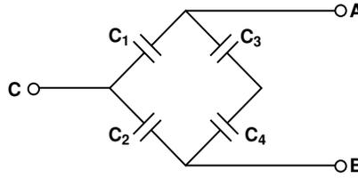
The equivalent adjacent capacitance is the capacitance between points A and C in the figure below. This capacitance is calculated using the following formula
