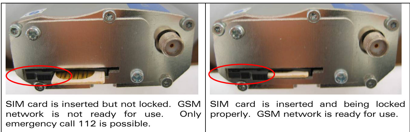
Figure 11: SIM card lock feature
