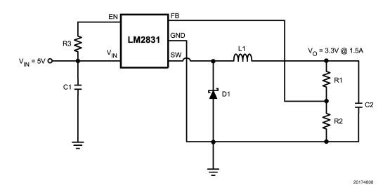
FIGURE 11. LM2831Z (3MHz): Vin = 5V, Vo = 3.3V @ 1.5A
