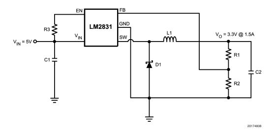
FIGURE 9. LM2831Y (550kHz): Vin = 5V, Vout = 3.3V @ 1.5A
