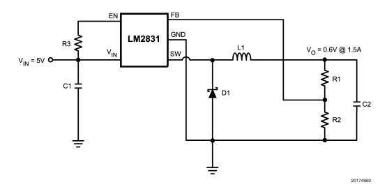
FIGURE 7. LM2831X (1.6MHz): Vin = 5V, Vo = 0.6V @ 1.5A
