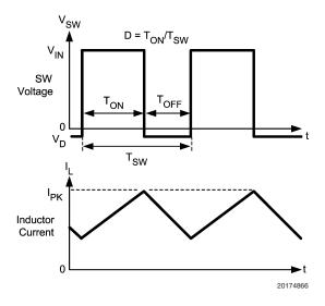
FIGURE 2. Typical Waveforms
