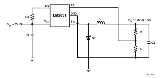
FIGURE 12. LM2831Z (3MHz): Vin = 5V, Vo = 1.2V @ 1.5A
