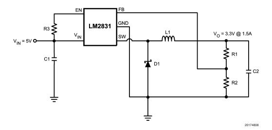
FIGURE 8. LM2831X (1.6MHz): Vin = 5V, Vo = 3.3V @ 1.5A
