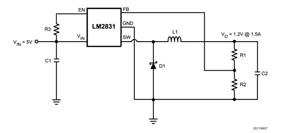
FIGURE 6. LM2831X (1.6MHz): Vin = 5V, Vo = 1.2V @ 1.5A
