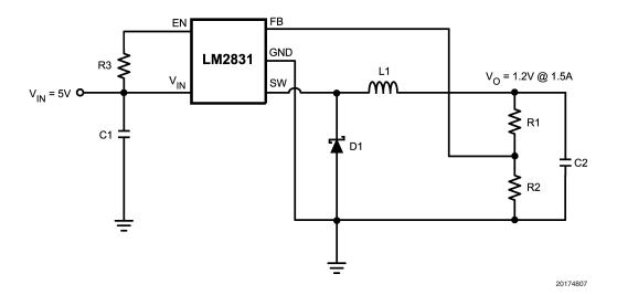
FIGURE 10. LM2831Y (550kHz): Vin = 5V, Vout = 1.2V @ 1.5A
