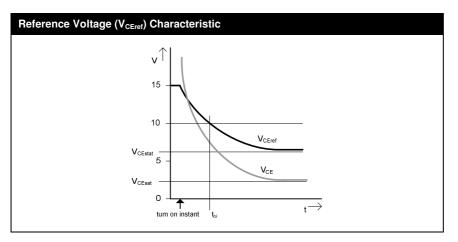
After  $t_{bl}$  has passed, the V<sub>CE</sub> monitoring will be triggered as soon as V<sub>CE</sub> > V<sub>CEref</sub> and will turn off the IGBT. The error memory will be set, and the output PRIM\_HOLD\_OUT changes to the HIGH state. Possible failure modes are shows in the following pictures.
