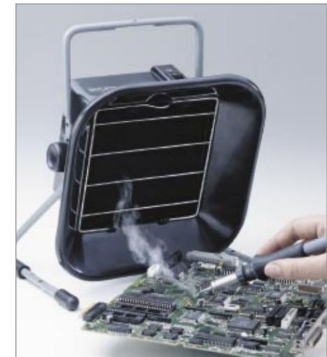
The Arm-Evac 50 is a unique, portable, cost-effective, bench-top fume extractor that provides wide area fume extraction or highly efficient source capture at up to two points using the optional arm attachment. The Arm-Evac 50 features operator adjustable airflow, quiet operation and a wide variety of filter options to meet the needs of virtually any application.
