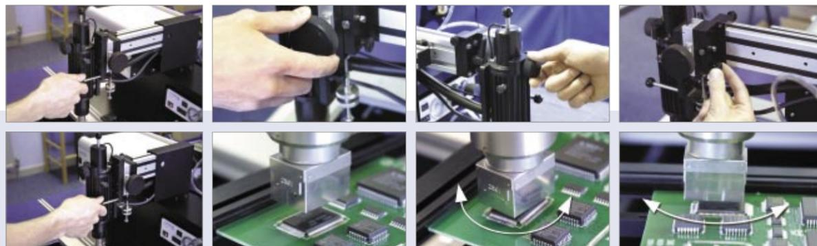
Reflow head moves back and out of the way to give you clear PCB access for board prep and clean up.
