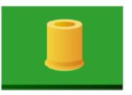
Solder the Mounting Pillar in place using standard surface mount Techniques
