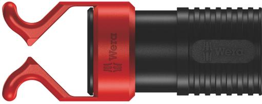
**Application:** Accessories with holding function for screws; fixes all screw profiles and sizes securely to the tool, suitable for round and hexagon blades with a diameter from 2.5 mm to 4.5 mm and 4.5 mm to 6 mm
