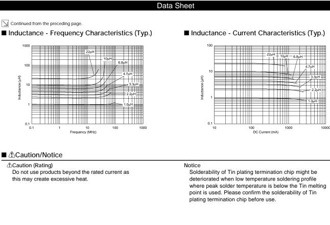
• This data sheet is applied for CHIP INDUCTORS (CHIP COILS) used for General Electronics equipment for your design.
