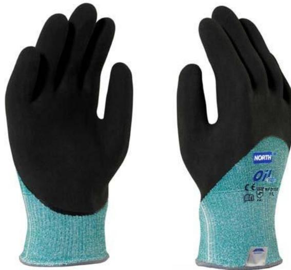
**Description:** Seamless Dyneema/glassfibre liner for highest cut protection according to level 5 as per EN388. This glove is treated with a special double dipped nitrile coating to make it oil repellent. The ideal combination for high finger sensitivity and still very high cut protection.
