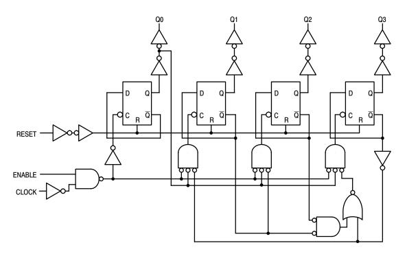
Figure 4. Decade Counter (MC14518B) Logic Diagram (1/2 of Device Shown)
