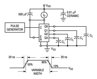
Figure 1. Power Dissipation Test Circuit and Waveform
