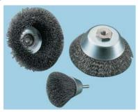
Filled with 30swg steel wire. Used for heavy duty cleaning of large metal surfaces. They remove weld scale, old paint and corrosion, and prepare metals to a good finish ready to accept paint treatment. The larger diameter brushes are manufactured with threaded bores to fit portable angle grinders etc.
