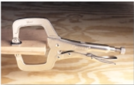
Locking C-Clamps allow quick, easy positioning of workpieces. Swivel tips minimize marring on softer materials.
