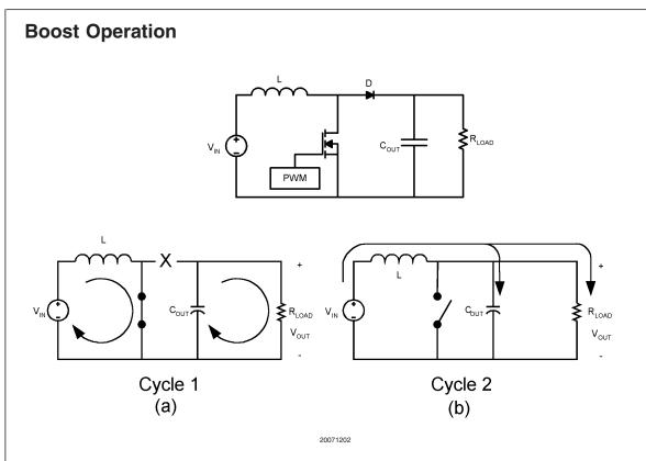
FIGURE 1. Simplified Boost Converter Diagram (a) First Cycle of Operation (b) Second Cycle Of Operation
