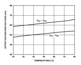
Figure 38. Output Saturation Voltage vs. Temperature
