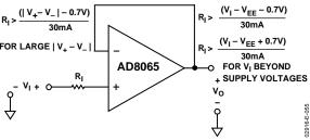
Figure 55. Current-Limiting Resistor
