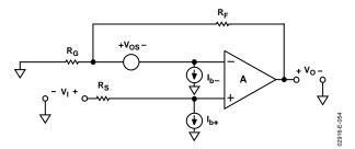
Figure 54. Voltage Feedback Amplifier DC Errors
