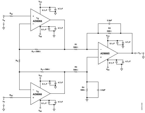
Figure 60. High Speed Instrumentation Amplifier
