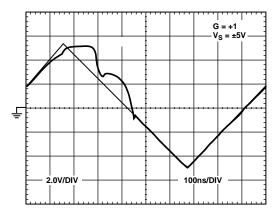
Figure 27. Input Overdrive Recovery (See Figure 42)
