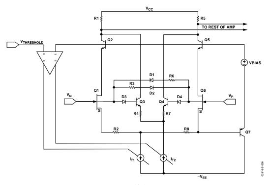
Figure 56. Simplified Input Stage
