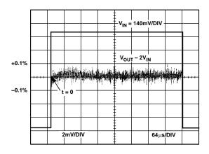
Figure 28. Long-Term Settling Time (See Figure 49)
