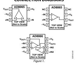
The AD8065/AD8066 are high performance, high speed, FET input amplifiers available in small packages: SOIC-8, MSOP-8, and SOT-23-5. They are rated to work over the industrial temperature range of  $-40^{\circ}$ C to  $+85^{\circ}$ C.
