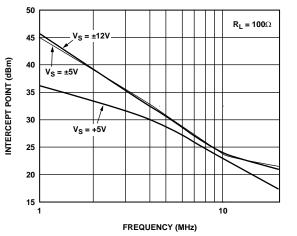
Figure 18. Third-Order Intercept vs. Frequency and Supply Voltage
