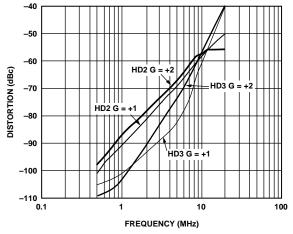
Figure 19. Harmonic Distortion vs. Frequency for Various Gains (See Figure 42 and Figure 43)
