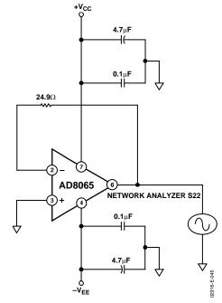
Figure 45. Output Impedance G = +1
