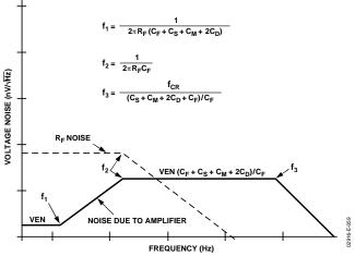
Figure 59. Photodiode Voltage Noise Contributions
