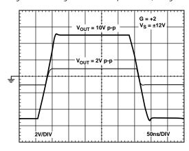
Figure 26. Large Signal Transient Response (See Figure 43)
