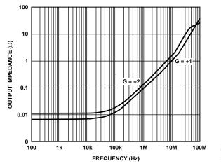
Figure 37. Output Impedance vs. Frequency (See Figure 45 and Figure 47)
