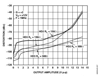
Figure 17. Harmonic Distortion vs. Amplitude for Various Loads  $V_S = \pm 12 V$  (See Figure 43)
