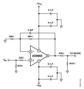
Figure 49. Settling Time
