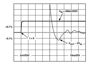
Figure 31. 0.1% Short-Term Settling Time (See Figure 49)
