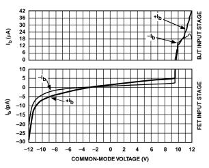
Figure 32. Input Bias Current vs. Common-Mode Voltage Range (See the Input and Output Overload Behavior Section)
