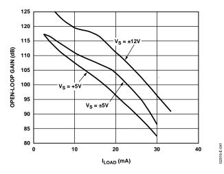
Figure 41. Open-Loop Gain vs. Load Current for Various Supply Voltages
