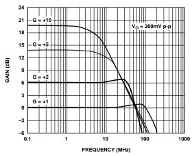
Figure 2. Small Signal Frequency Response
