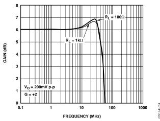
Figure 14. Small Signal Frequency Response for Various R<sub>LOAD</sub> (See Figure 43)
