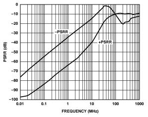
Figure 36. PSRR vs. Frequency (See Figure 48 and Figure 50)
