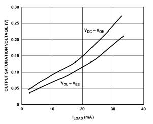
Figure 35. Output Saturation Voltage vs. Output Load Current
