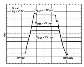
Figure 23. Large Signal Transient Response (See Figure 42)
