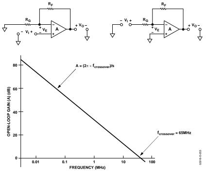
Figure 53. Open-Loop Gain vs. Frequency and Basic Connections
