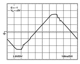
Figure 24. Output Overdrive Recovery (See Figure 44)
