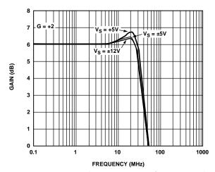
Figure 9. Large Signal Frequency Response for Various Supplies (See Figure 43)
