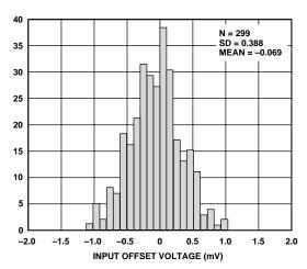
Figure 33. Input Offset Voltage
