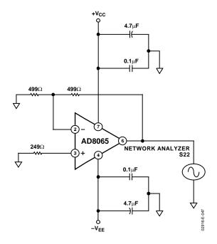
Figure 47. Output Impedance G = +2
