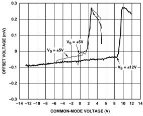
Figure 30. Input Offset Voltage vs. Common-Mode Voltage
