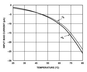
Figure 29. Input Bias Current vs. Temperature
