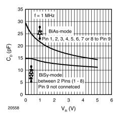
Figure 3. Typical Capacitance C<sub>D</sub> vs. Reverse Voltage V<sub>R</sub>
