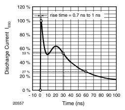
Figure 2. ESD Discharge Current Wave Form acc. IEC 61000-4-2 (330 Ω/150 pF)
