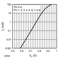
Figure 4. Typical Forward Current I<sub>F</sub> vs. Forward Voltage V<sub>F</sub>
