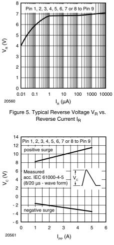
Figure 6. Typical Peak Clamping Voltage V\_C vs. Peak Pulse Current  $\rm I_{PP}$
